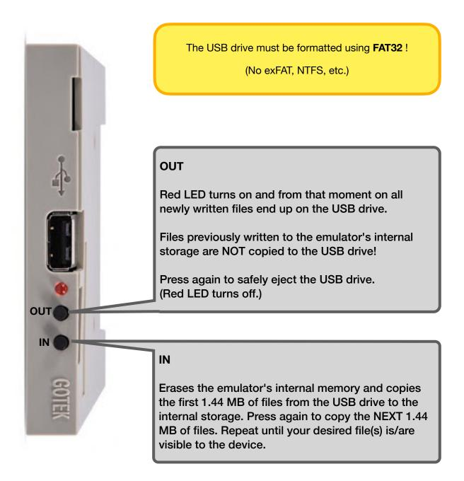
The GOTEK SFR1M44-DU26 has an internal storage of 1.44 MB. If no USB drive is connected, this internal storage is visible to and usable by the device. I.e. you can write files to it and read them again. BUT: There's no way to copy files from that internal storage to a USB drive.
